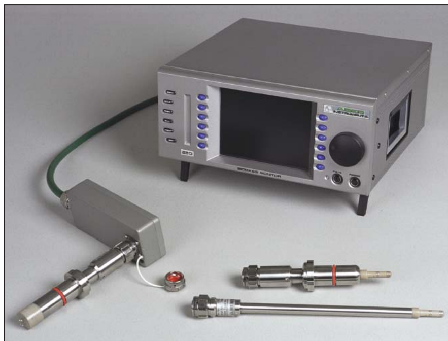
Figure 2. The Aber Biomass Monitor model 220; suitable for frequency scanning.
